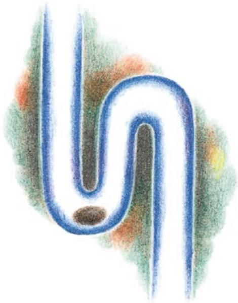
Over time, debris traveling through the pipes may collect in a bend. Debris that collects and restricts water flow is known as a clog or a blockage.
