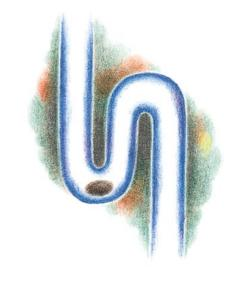
Over time, debris traveling through the pipes may collect in a bend. Debris that collects and restricts water flow is known as a clog or a blockage.
